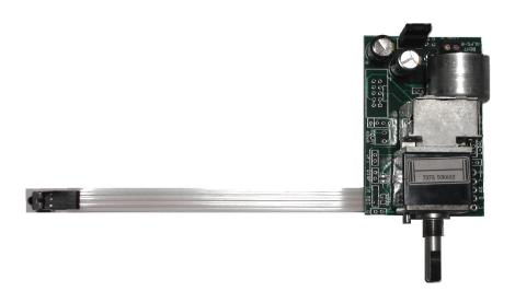
This document describes the wiring and required space of the Bent Audio Remote ALPS potentiometer board. This is a good choice where the cost or complexity of a stepped or relay based attenuator is too high. The PCB comes with the remote handset and it is all completely assembled and tested – just power up and you are ready to go.
